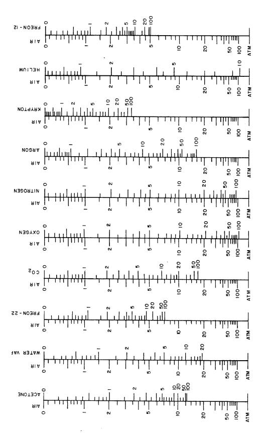
NOMOGRAM SHOWING CALIBRATION OF HASTINGS VACUUM GAUGES WHICH USE THE DV-100 GAUGE TUBES FOR THE GASES SHOWN ABOVE. TO FIND THE PRESSURE IN A GAS OTHER THAN AIR, LOCATE THE OBSERVED READING ON THE "AIR" SIDE OF THE APPROPRIATE SCALE AND READ, ON THE OPPOSITE SIDE OF THE SCALE. THE TRUE PRESSURE IN MICRONS OF MERCURY FOR THE GAS BEING MEASURED.
